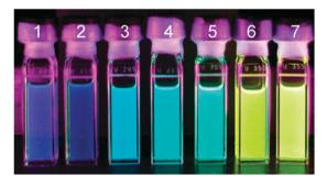
Light-driven modulation of fluorescence color from azobenzene derivatives containing electron-donating and electron-withdrawing groups
